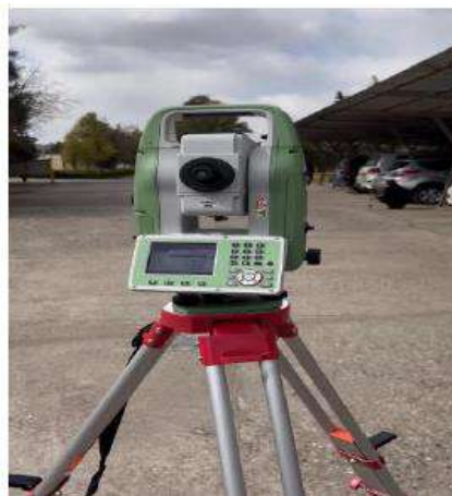
Figure (4-6) Total station setup
