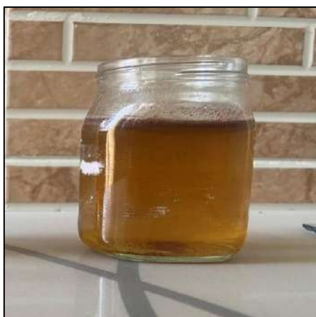
Figure 4.15 PP in 15% HCl solution after the reaction time
