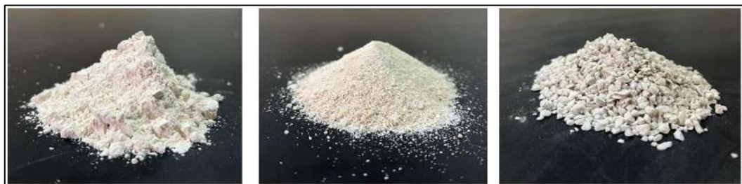
Figure 3.1 Fine, medium and coarse sized of \text{CaCO}_3 LCM
