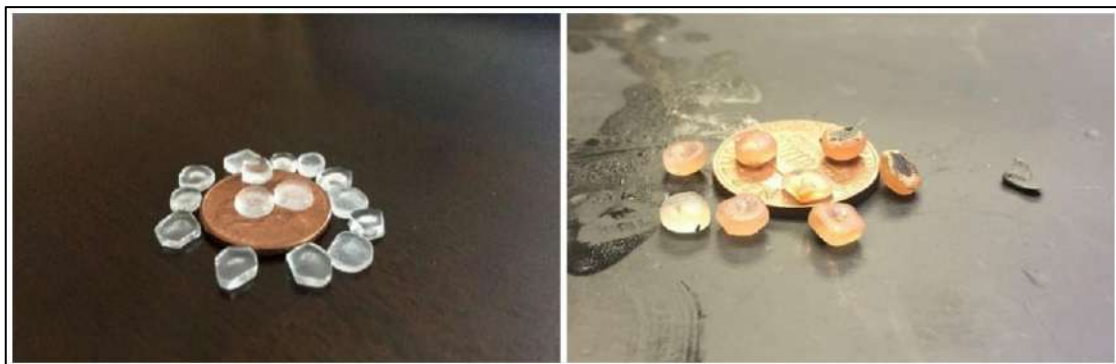
Figure 2.13 The novel smart LCM before being activated (left) and after being activated (right) (Mansour et al., 2019).
