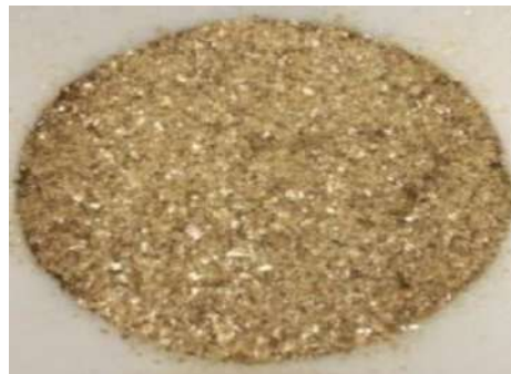
Figure 2.9 Mica flaky material (Alsaba et al. 2014)
