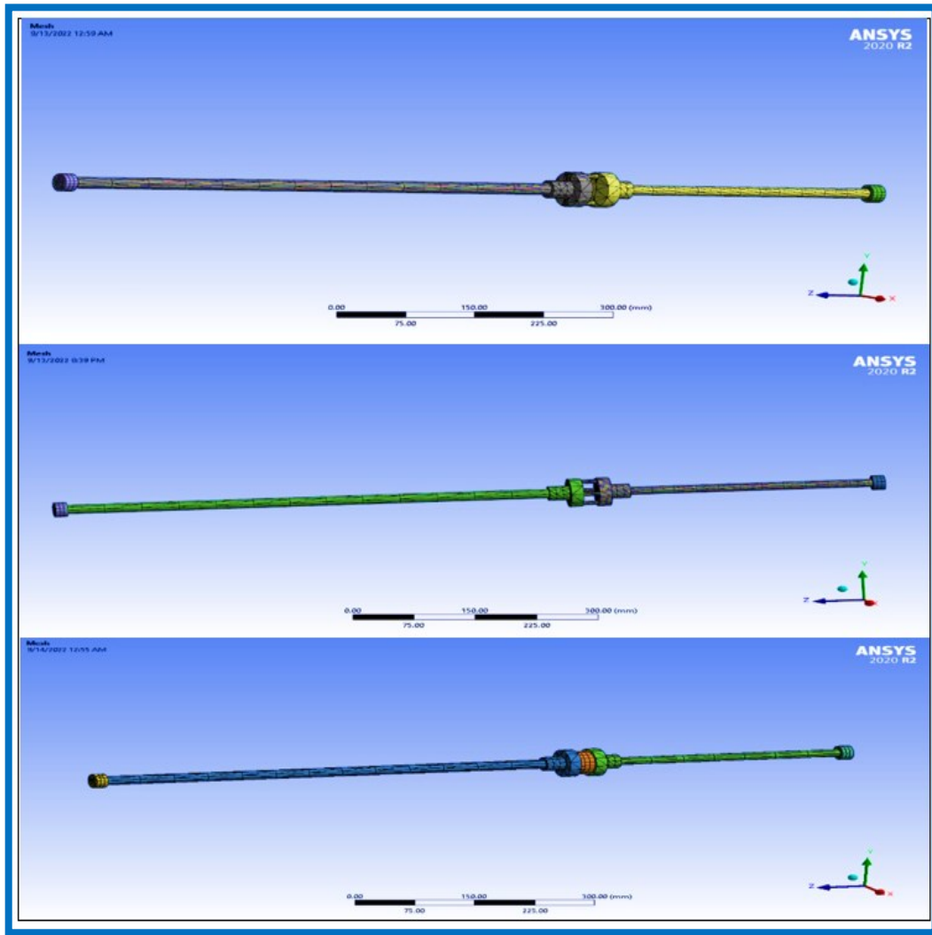
Fig. 9: The automatic mesh using to mesh the structural model of the system.
