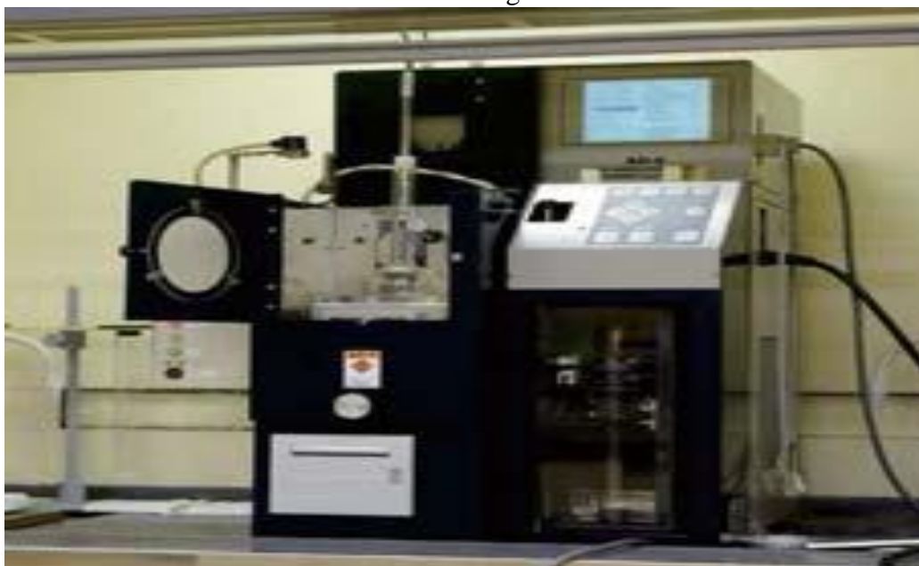
Figure 1. Automatic distillation tower
